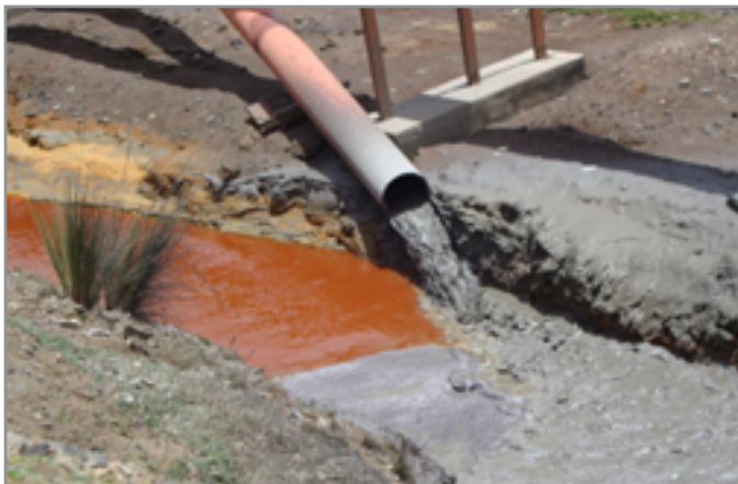
Wet tailings disposal at a mine in Peru PHOTO: Centro de Cultura Popular LABOR, Peru
